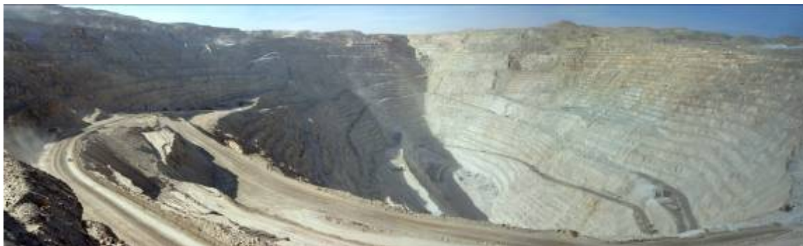
Panorama of the pit at Chuquicamata. 9.5 km to the end , 6.1 km across, and 1050 m down the wall!
